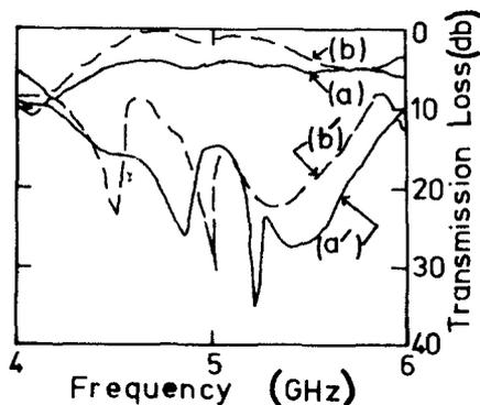
Figure 8 Performance of an edge-guided mode isolator at an applied field of 0.1250 T: (a) and (b) total insertion loss, (a') and (b') isolation.
