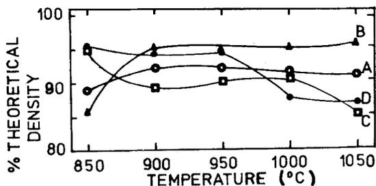
Figure 4 Percentage of theoretical density plotted as a function of sintering temperature for a sintering time of 6 h for lithium ferrite containing: (a) 1 wt%  $\text{Bi}_2\text{O}_3$ , (b) 2 wt%  $\text{Bi}_2\text{O}_3$ , (c) 4 wt%  $\text{Bi}_2\text{O}_3$  and (d) 7 wt%  $\text{Bi}_2\text{O}_3$ .
