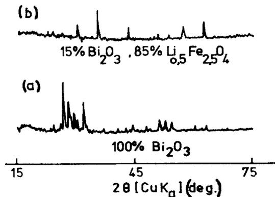
Figure 5 X-ray diffraction pattern of (a)  $\text{Bi}_2\text{O}_3$  and (b) 85 wt%  $\text{Li}_{0.5}\text{Fe}_{2.5}\text{O}_4$  - 15 wt%  $\text{Bi}_2\text{O}_3$  heated at  $950^\circ\text{C}$  for 6 h.
