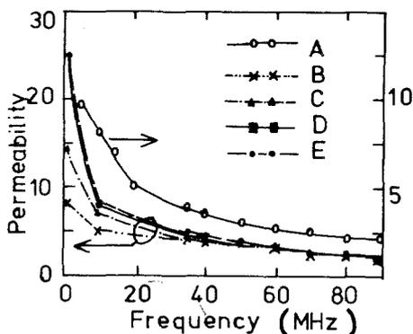
Figure 7 Variation of initial permeability as a function of frequency for (A) 0 wt%  $Bi_2O_3$ , (B) 1 wt%  $Bi_2O_3$ , (C) 2 wt%  $Bi_2O_3$ , (D) 4 wt%  $Bi_2O_3$  and (E) 7 wt%  $Bi_2O_3$ .
