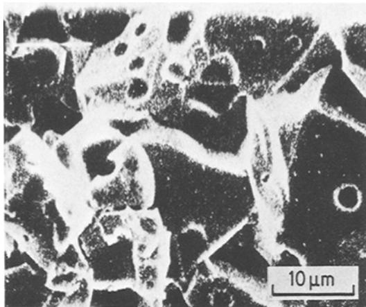
Figure 3 SEM fractograph of 98 wt%  $\text{Li}_{0.5}\text{Fe}_{2.5}\text{O}_4$  - 2 wt%  $\text{Bi}_2\text{O}_3$ , heated at  $950^\circ\text{C}$  for 6 h.
