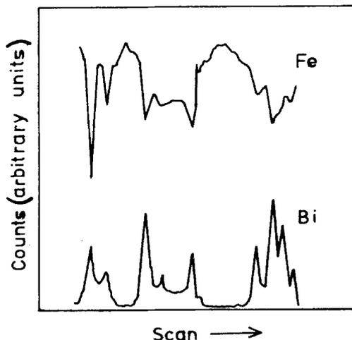
Figure 6 EPMA distribution of iron and bismuth in 85 wt%  $\text{Li}_{0.5}\text{Fe}_{2.5}\text{O}_4$  - 15 wt%  $\text{Bi}_2\text{O}_3$  heated at  $950^\circ\text{C}$  for 6 h.
