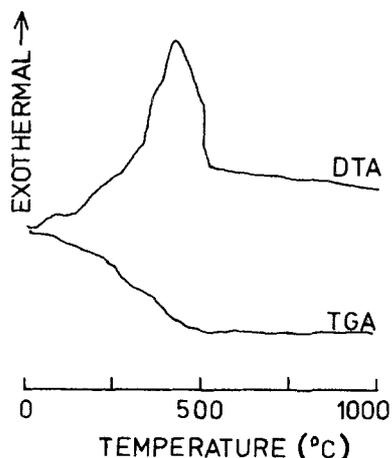
Figure 1 DTA and TGA curves for the mixture of organometallic complex at a heating rate of  $10^{\circ}\text{C min}^{-1}$ .
