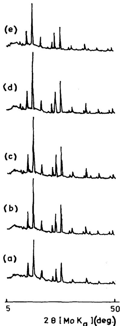
Figure 2 X-ray diffraction pattern of the mixture of organometallic complex heated at: (a)  $800^{\circ}\text{C}$  for 0.5 h, (b)  $800^{\circ}\text{C}$  for 1 h, (c)  $800^{\circ}\text{C}$  for 2 h, (d)  $800^{\circ}\text{C}$  for 4 h and (e)  $420^{\circ}\text{C}$  for 4 h.
